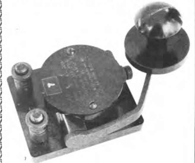
● (7) J-5-A. USA Signal Corps, WW-2 (Flame Proof key) 1941.
